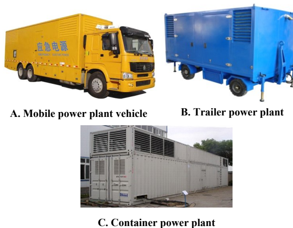
Fig. 2. Different types of mobile power source
